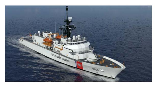
The notional OPC design is 360 feet long, with a beam of 54 feet and a draft of 17 feet. Graphic courtesy of Eastern Shipbuilding Group.
