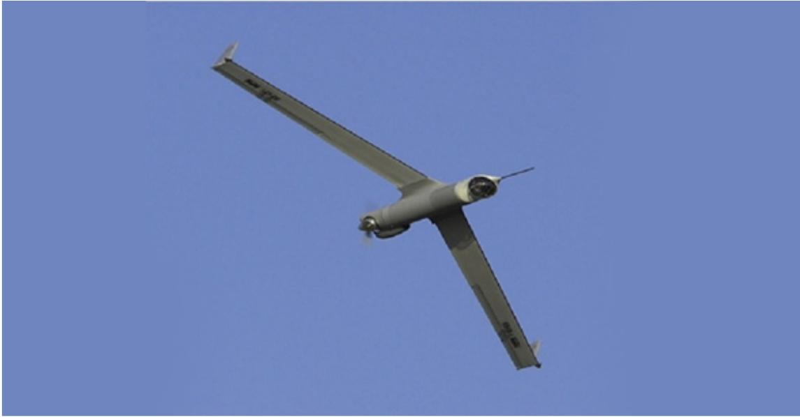
The ScanEagle sUAS will augment the national security cutter's embarked manned helicopter capability with 12 hours of continuous flight time and up to 200 hours of on-station sensor data per month. Courtesy photo.
