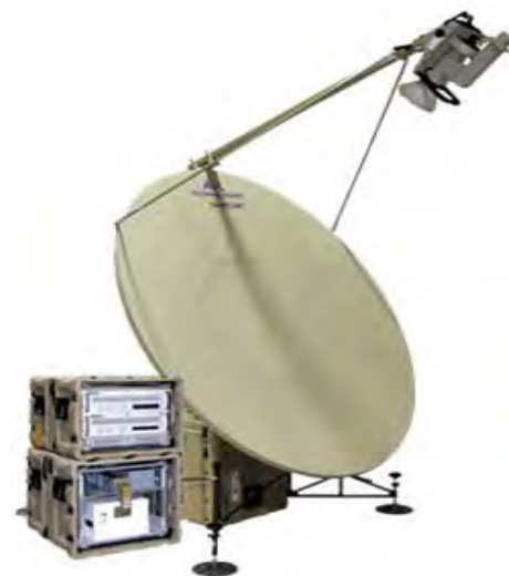
The new Troposcatter equipment is provided through a CRADA with ComTech Systems.
