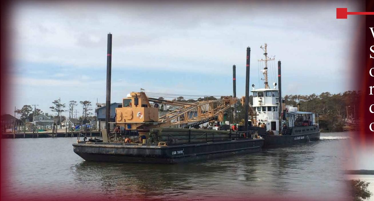
WLICs such as Coast Guard Cutter Smilax usually carry 20 to 30 pilings on each discrepancy response trip to replace ATON destroyed by natural disasters, damage from ships, or erosion over time.
