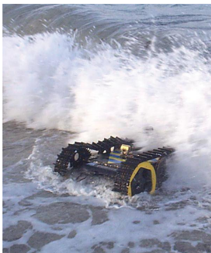
C-TAR/C-TALON. Primarily in response to the inability to land forces in a direct beach assault in Desert Storm, a swarm of six TAR-class robots were waterproofed and instrumented for mine detection and neutralization (DARPA, 2010a).
