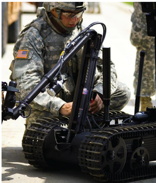
TALON III-These 100-lb robots, developed for EOD applications, are successfully used to counter IEDs in military theaters of operations saving many EOD technicians' lives. Today over 3,000 are currently used by the military (DARPA, 2010a).
