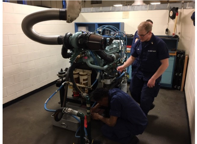
Naval Engineers from CGA Class of 2019 prepare a diesel engine to conduct valve lash check and adjustments.
