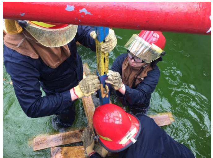
Naval Engineers from CGA Class of 2019 erect mechanical shoring to combat simulated damage to a hatch.
