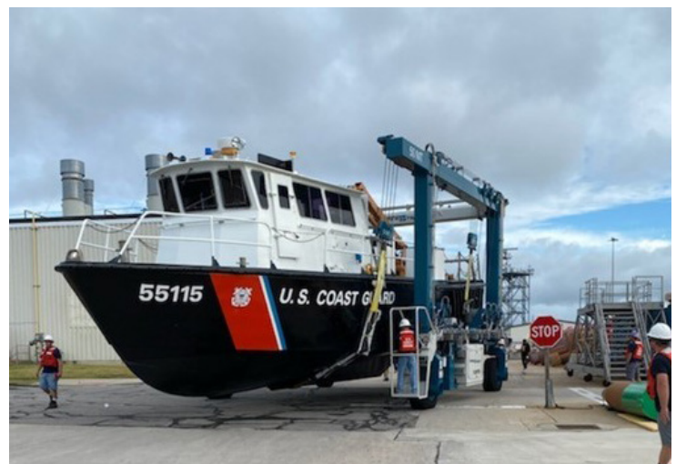
CG 55115 being transported by IPF Portsmouth's mobile boat hoist after completion of the drydock package.
