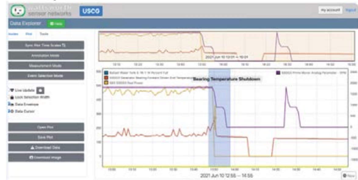
Figure 1: Wattsworth Sensor Networks Monitoring a Bearing Temperature Shutdown from SSDG3
