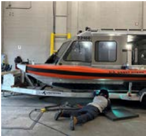
Weld repairs in process on assets
