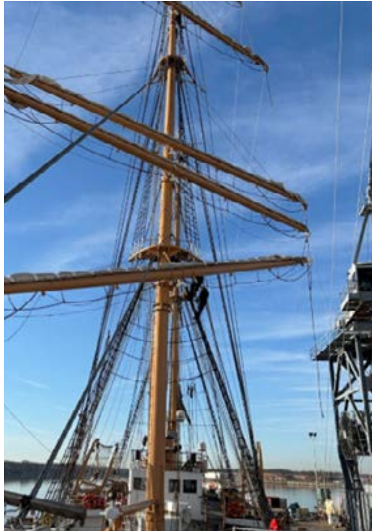
EAGLE Main Mast After a Comprehensive Overhaul
