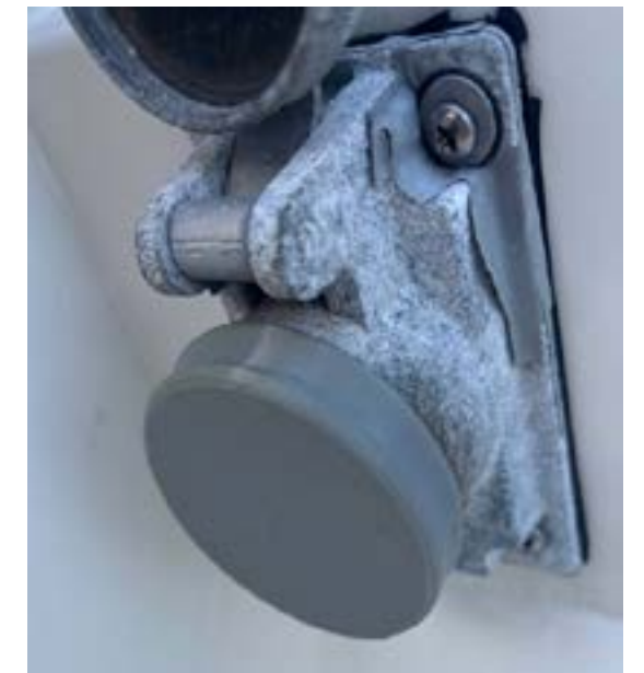
3D Printed replacement cap
