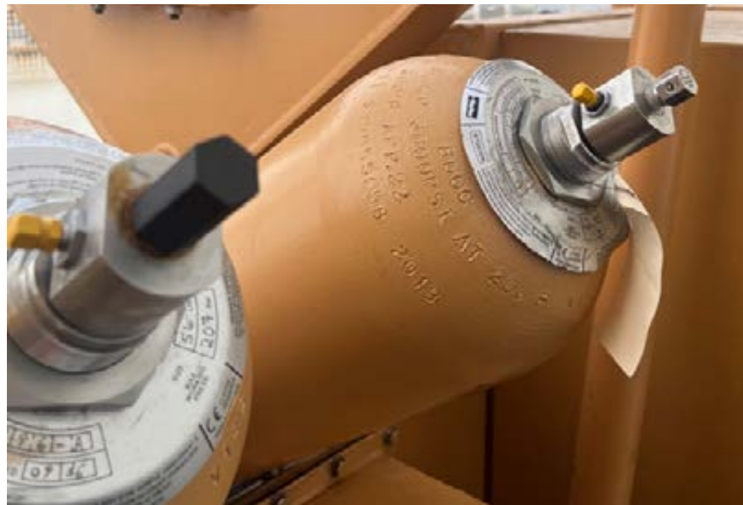
One covered Welin Lambie Accumulator w/ 3D printed replacement and one open to the elements, awaiting a cover.
