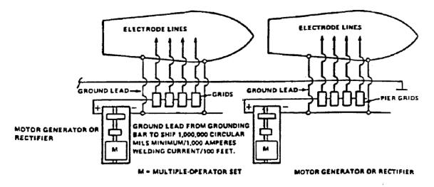
NOTE: WELDING ON TWO OR MORE SHIPS (IN CASE OF MULTIPLE-OPERATOR MACHINE) SHOULD NOT BE PERFORMED WITH THE SAME GENERATOR OR RECTIFIED.
