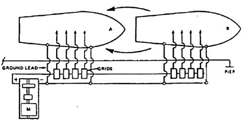
NOTE: WHEN TWO SHIPS ARE CONNECTED TO THE SAME GENERATOR OR RECTIFIER, THE RESISTANCE OF THE NEGATIVE RETURN BETWEEN THE SHIPS CANNOT BE MADE LOW IN COMPARISON WITH THE RESISTANCE THROUGH THE WATER. SOME OF THE CURRENT USED ON SHIP & FLOWS THROUGH THE WATER, CORRODING METAL OFF SHIP & AND POSSIBLY BLISTERING PAINT ON SHIP A.
