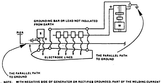
FLOWS FROM THE SHIPS HULL TO THE WATER AND EVENTUALLY REACHES THE NEGATIVE SIDE OF THE GENERATOR OR RECTIFIER.
