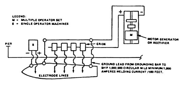
NOTE: GROUNDING BAR OR LEAD SHALL BE INSULATED FROM EARTH AND OTHER STRUCTURES, BE OF SUFFICIENT CROSS-SECTIONAL AREA TO CARRY THE WELDING CURRENT, AND SHOULD REMAIN ABOVE WATER WITH TIDE CHANGES OR SHIP MOVEMENTS.
