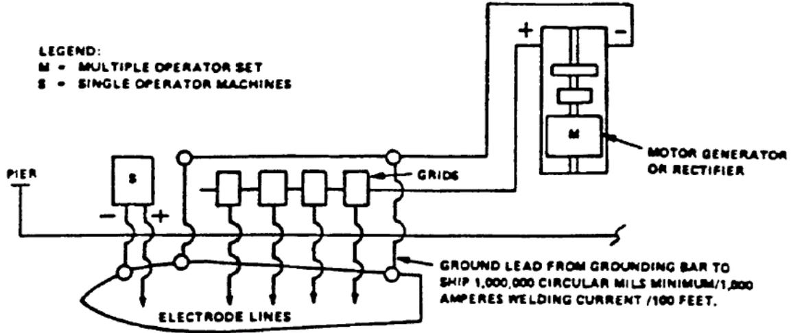
**NOTE:** GROUNDING BAR OR LEAD SHALL BE INSULATED FROM EARTH AND OTHER STRUCTURES, BE OF SUFFICIENT CROSS-SECTIONAL AREA TO CARRY THE WELDING CURRENT, AND SHOULD REMAIN ABOVE WATER WITH TIDE CHANGES OR SHIP MOVEMENTS.
