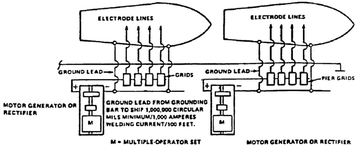
NOTE: WELDING ON TWO OR MORE SHIPS (IN CASE OF MULTIPLE-OPERATOR MACHINE) SHOULD NOT BE PERFORMED WITH THE SAME GENERATOR OR RECTIFIER.
