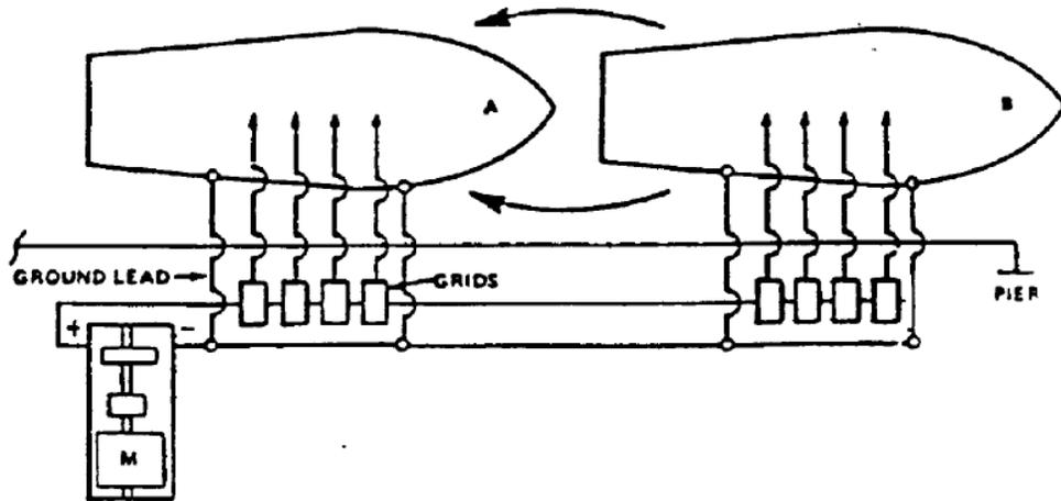
NOTE: WHEN TWO SHIPS ARE CONNECTED TO THE SAME GENERATOR OR RECTIFIER, THE RESISTANCE OF THE NEGATIVE RETURN BETWEEN THE SHIPS CANNOT BE MADE LOW IN COMPARISON WITH THE RESISTANCE THROUGH THE WATER. SOME OF THE CURRENT USED ON SHIP B FLOWS THROUGH THE WATER, CORRODING METAL OFF SHIP B AND POSSIBLY BLISTERING PAINT ON SHIP A.
