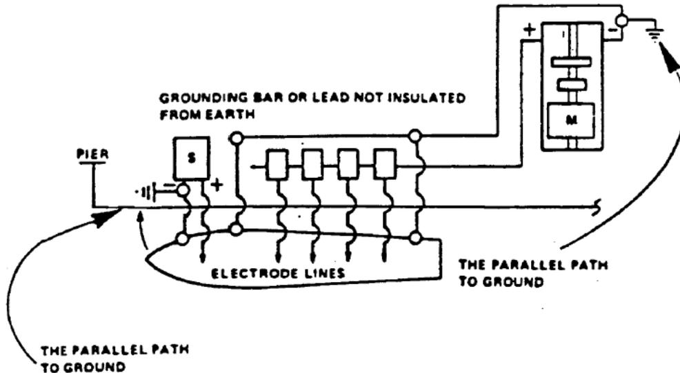
**NOTE:** WITH NEGATIVE SIDE OF GENERATOR OR RECTIFIED GROUNDED, PART OF THE WELDING CURRENT FLOWS FROM THE SHIP'S HULL TO THE WATER AND EVENTUALLY REACHES THE NEGATIVE SIDE OF THE GENERATOR OR RECTIFIER.
