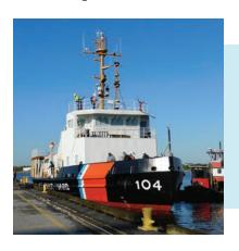
CGC BISCAYNE BAY, a 140' Bay Class Icebreaking Tug (WTGB), at the completion of its Service Life Extension Program (SLEP). The Bay Class were built between 1979 and 1988. The last WTGB completed SLEP in Fiscal Year (FY) 2020, ensuring an additional 15 years of domestic icebreaking capability in the Northeast and Great Lakes.
