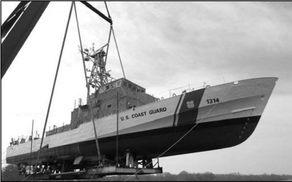
*Riggers at the Yard return the Coast Guard Cutter SAPELO to sea to begin the final phase of the patrol boat's modernization in April, 2011. Upon completion of work at the shipyard, SAPELO returned to its homeport in San Juan, Puerto Rico, to support Coast Guard operational missions.*
