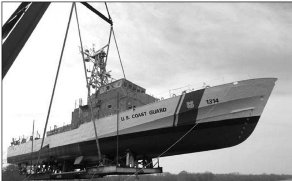
*Riggers at the Yard return the Coast Guard Cutter SAPELO to sea to begin the final phase of the patrol boat's modernization in April, 2011. Upon completion of work at the shipyard, SAPELO returned to its homeport in San Juan, Puerto Rico, to support Coast Guard operational missions.*
