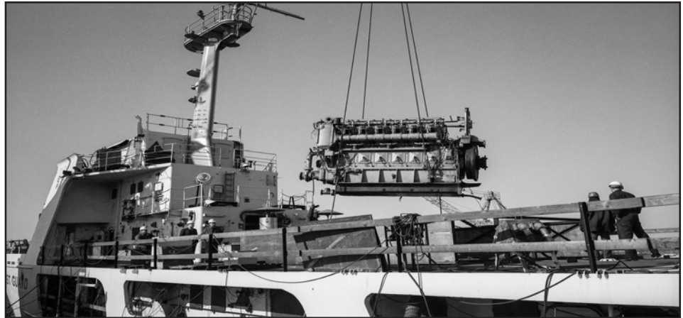
Yard workers conduct a mid-life overhaul of the Coast Guard Cutter ACTIVE in 1984, the first of fourteen 210' medium endurance cutters to receive an extensive facelift under the 210' Major Maintenance Availability program that concluded in 1998.
