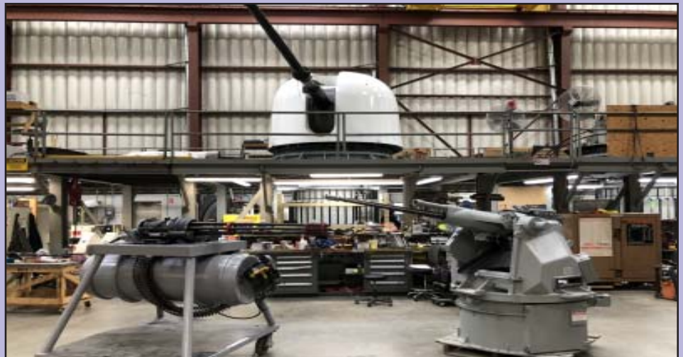
National Security Cutter’s 20mm Close-In-Weapon System (left); Fast Response Cutter’s MK38 Mod 2 25mm Machine Gun (right); High & Medium Endurance Cutter’s MK75 76mm Gun (center)
