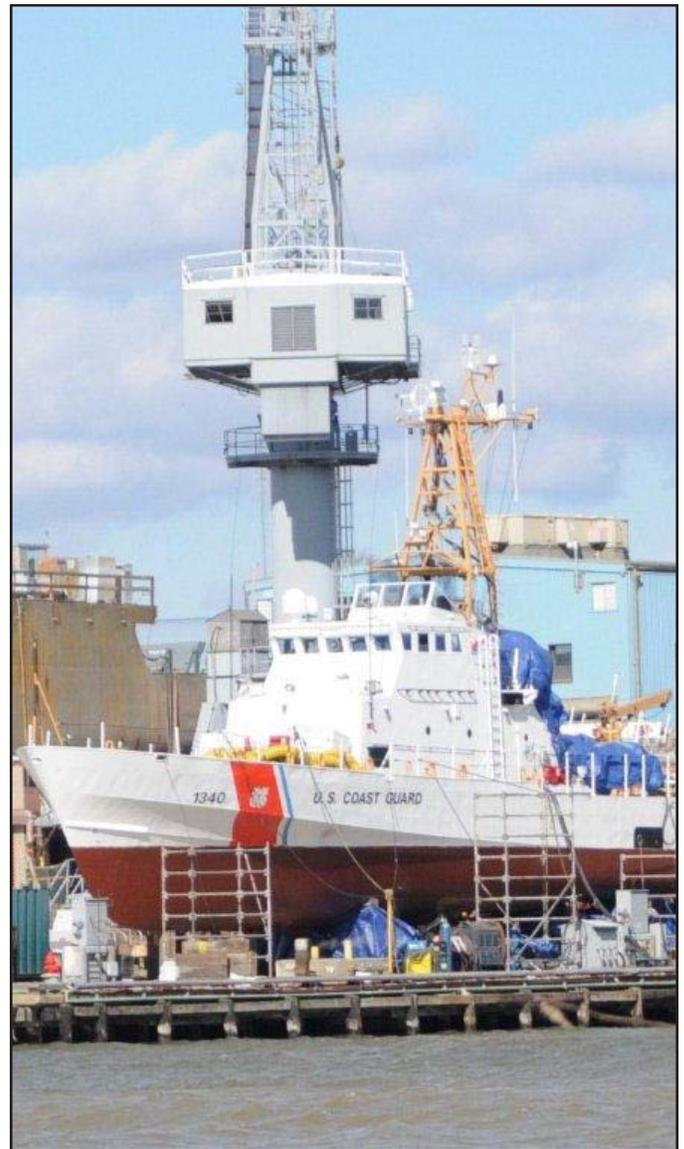
*The 110' patrol boat JEFFERSON ISLAND docks on the Yard's shiplift in January 2013 to undergo critical repairs.*
