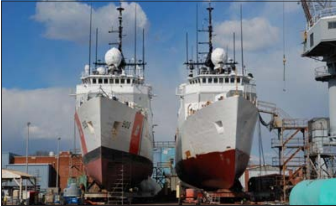
The Cutters SPENCER (WMEC 905), left, and CAMPBELL (WMEC 909), right, are currently dry-docked on the Yard's shiplift for modernization under the 270' Phase II Mission Effectiveness Project.
