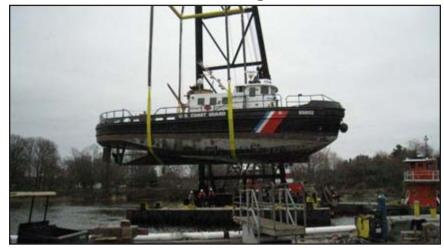
The Yard lifted the Cutter CHOCK on April 8<sup>th</sup> to begin an anticipated 10-week repair availability for routine maintenance. Additional work items include complete remediation of lead and asbestos in the aft steering and aft cargo hold compartment; structural work; painting of the underwater hull; removal/renewal of stern tube, and removal/reinstallation of two ship
