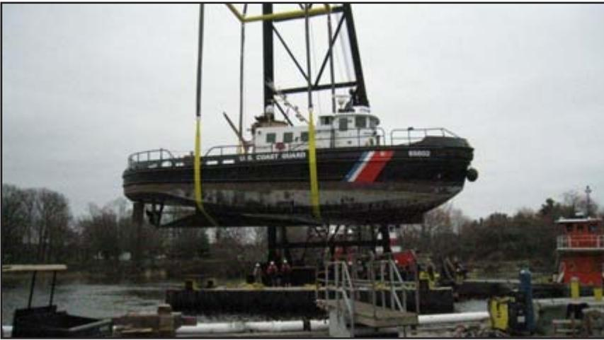
The Yard lifted the Cutter CHOCK on April 8<sup>th</sup> to begin an anticipated 10-week repair availability for routine maintenance. Additional work items include complete remediation of lead and asbestos in the aft steering and aft cargo hold compartment; structural work; painting of the underwater hull; removal/renewal of stern tube, and removal/reinstallation of two ship
