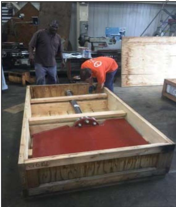
The Yard Structural and Mechanical Groups recently wrapped up a production project spanning the last three years that resulted in the fabrication of 66 rudders and shafts for the Coast Guard's 65' and 75' cutter fleets. Tradesmen in the Shipfitting, Welding, Woodworking, Paint and Inside Machine Shops procured materials, crafted, machined, painted and crated 26 propulsion shafts, 24 steering rudders, and 16 flanking rudders with a total dollar value of \$2.6 million.
