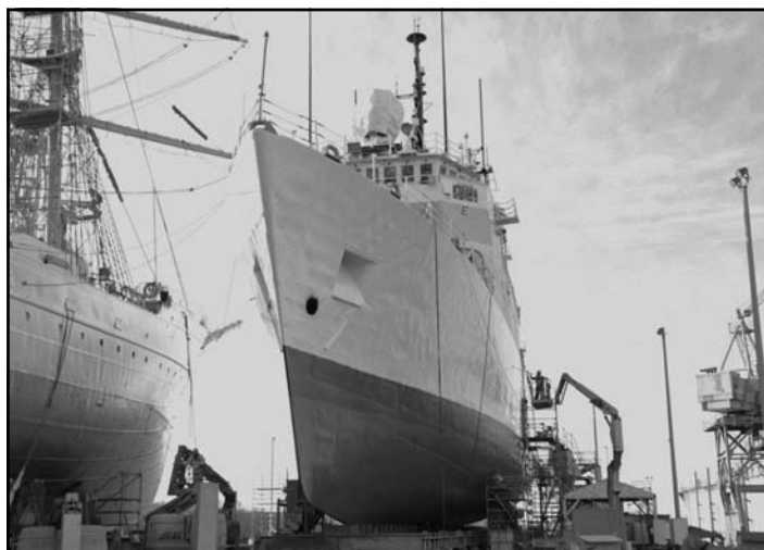
The Cutter BEAR dry-docks on the Yard's shiplift in December 2011 while undergoing the 270' Phase II MEP. BEAR is one of six 270' cutters overhauled at the Yard to date under the modernization project that is designed to replace aging systems on board select ships to improve reliability, reduce operating costs, and meet required mission hours.
