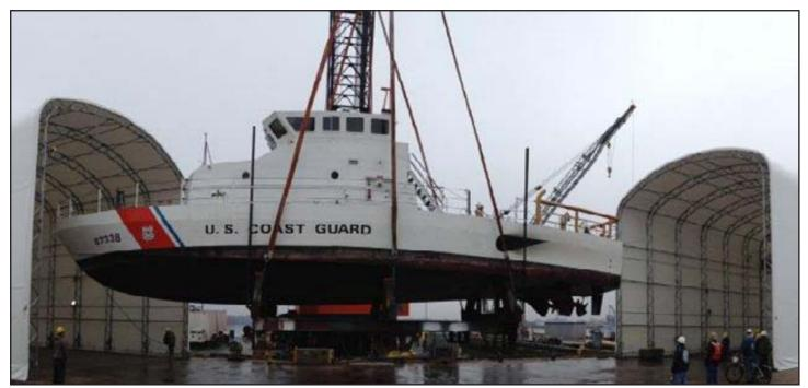
The 87' patrol boat IBIS is lifted into a tented dry-dock under the new 87' "bow-to-stern" project. The program uses a two-piece plastic wrapped scaffolding system for cutter repair, controlling weather conditions to support work schedules. When the boat is in place, two separate scaffold peices join together as one enclosed work space. The Yard has two tented scaffold systems on the waterfront to accommodate simultaneous "bow-to-stern" maintenance.
