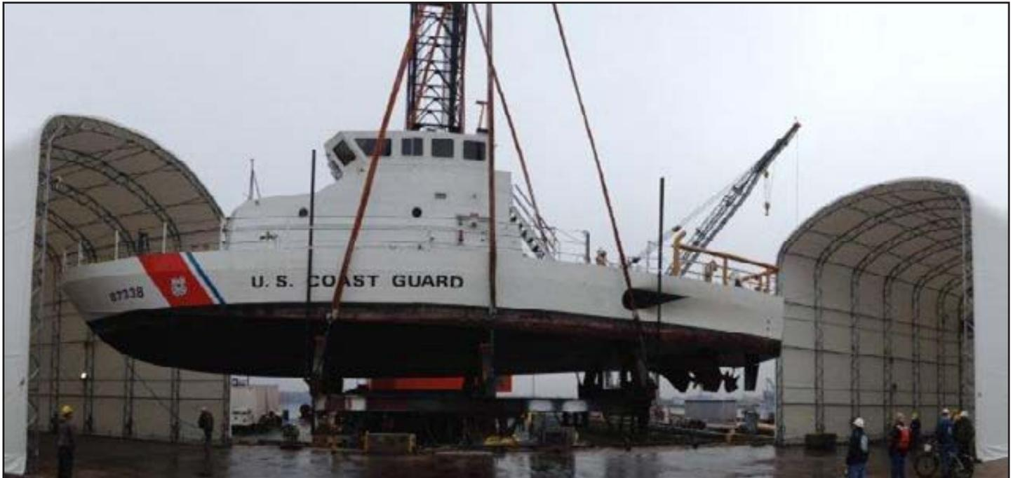
*The 87' patrol boat IBIS is lifted into a tented dry-dock under the new 87' "bow-to-stern" project. The program uses a two-piece plastic wrapped scaffolding system for cutter repair, controlling weather conditions to support work schedules. When the boat is in place, two separate scaffold pieces join together as one enclosed work space. The Yard has two tented scaffold systems on the waterfront to accommodate simultaneous "bow-to-stern" maintenance.*
