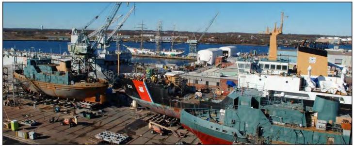
A snapshot of the Coast Guard's In-Service Vessel Sustainment (ISVS) Project throughout 2015 is featured with four ISVS cutters on the Yard's waterfront. Left to right on the shiplift are: 140' BRISTOL BAY; 225' OAK; 140' PENOBSCOT BAY. Barque EAGLE is pictured pier side in the background (center). The Yard completed ISVS overhaul on the first selected 140' icebreaking tug, MORRO BAY, in August 2015.
