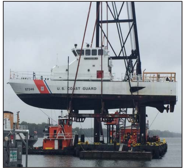
The Yard lifted the Cutter FLYINGFISH on September 30, 2016 to begin a 60-day planned maintenance on the patrol boat under the 87' Bow-To-Stern Program. FLYINGFISH was the 25th vessel in the repair project that includes a standardized work package, specialized infrastructure and equipment, and use of crew swaps between arriving and newly delivered cutters. The Yard completed FLYINGFISH on November 30th - on time and under budget. The patrol boat is homeported in Virginia Beach, VA. (Photo by LCDR Miles Randall)
