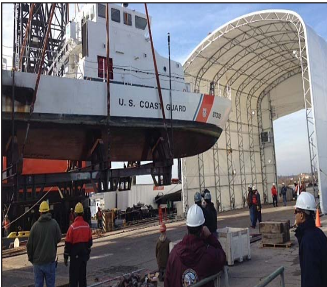
The 87' patrol boat BLUEFIN departs the tented, plastic wrapped scaffolding system concluding a 60-day planned maintenance under the Coast Guard's 87' Bow-To-Stern (BtoS) project. Work throughout the repair period was accomplished irregardless of outside weather conditions. (Photo by LCDR Miles Randall)
