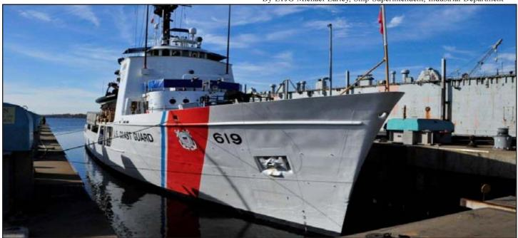
The 210' medium endurance cutter CONFIDENCE arrived at the Yard on November 18th for a rapid three-week emergency dry dock availability. The cutter crew had recently identified excessive corrosion and wastage in the engine room bilge prior to deployment on an operational patrol from its homeport in Cape Canaveral, Florida.
