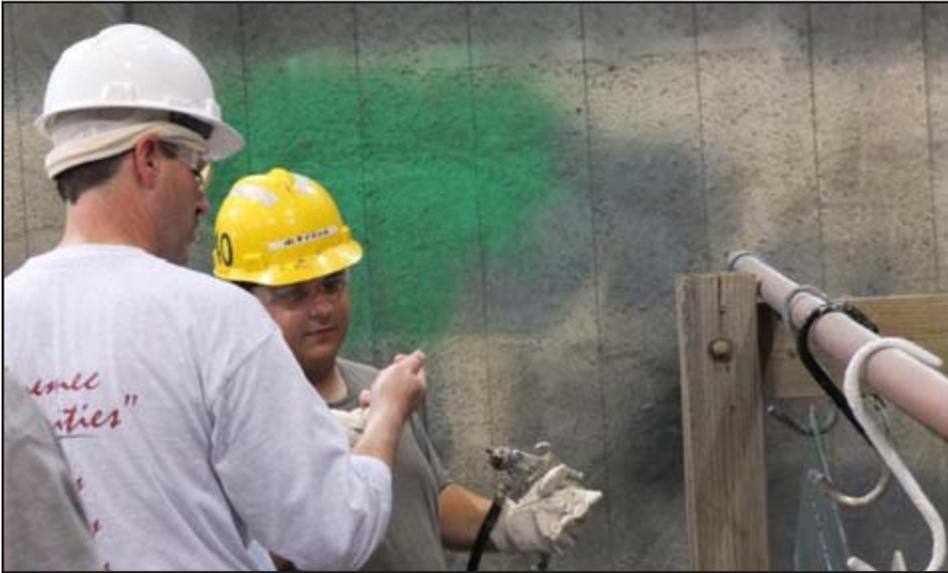
*A NACE instructor (center) demonstrates measurement of wet film thickness of marine coating 302h zinc (a modified organic zinc) to Yard paint trade theory trainee, William Bittner, Jr. (right).*
