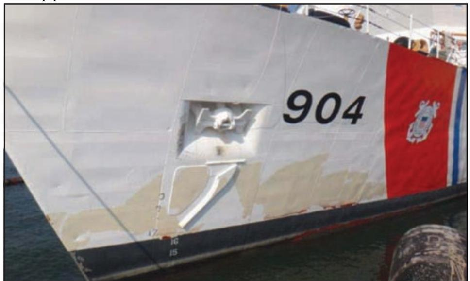
*The 270’ medium endurance cutter NORTHLAND underwent modernization as a Mission Effectiveness Project (MEP) from April 2010 to March 2011. As part of the MEP contract, painting and coatings of the cutter’s underwater hull, body, and freeboard took place. As evidenced in the photo above, NORTHLAND reported paint failure to the port side, forward freeboard, boot-top and underwater hull in May 2011.*
