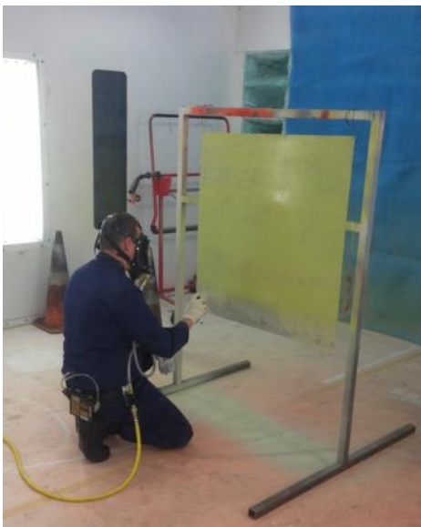
Primer application inside paint booth
