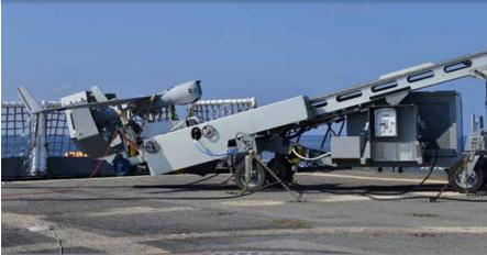
ScanEagle UAS deployed on Coast Guard Cutter Stratton. The ScanEagle UAS has a flight time of 18+ hours with a maximum speed of 96 miles per hour. U.S. Coast Guard photo by Petty Officer 1st Class Mark Barney.
