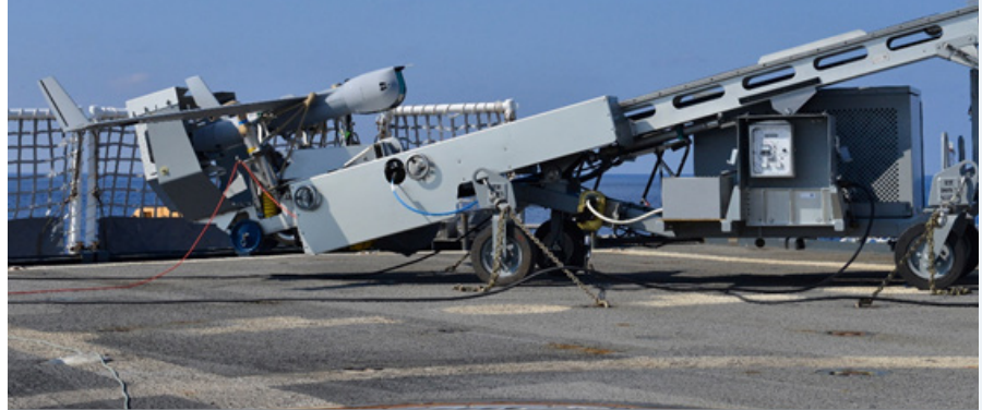
ScanEagle UAS deployed on Coast Guard Cutter Stratton. The ScanEagle UAS has a flight time of 18+ hours with a maximum speed of 96 miles per hour. U.S. Coast Guard photo by Petty Officer 1st Class Mark Barney.
