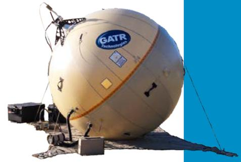
Using ground antennas, like the one shown here, Coast Guard researchers explored deployable satellite communications.
