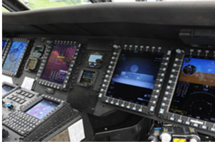
The MH-60T Jayhawk features a Common Avionics Architecture System (CAAS) “glass” cockpit, comprised of five multi-function displays that present a variety of information to the aircrew. In addition to the new avionics, the MH-60T also features an electro-optical/infrared sensor system and other life-saving equipment. U.S. Coast Guard photo by Petty Officer 3rd Class Charly Hengen.
