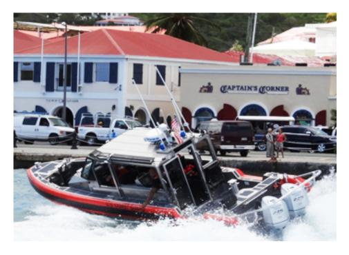
Coast Guard Sector San Juan, Puerto Rico, tests out one of four new Response Boat-Small (RB-S) II, delivered April 8–11. The new RB-S II gives Coast Guard operators upgraded electronics and communications, improved crew comfort to reduce fatigue, and improved visibility. U.S. Coast Guard photo by Lt. Nicholas Schellman.
