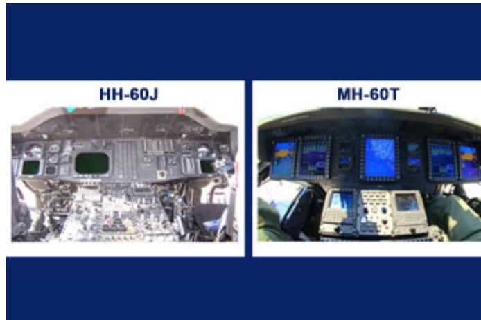
The cockpit of the MH-60T model (right) has been enhanced from the legacy HH-60J model (left), including installation of five multi-function displays showing flight instrument data, weather radar information, forward-looking infrared and camera imagery and an integrated traffic collision avoidance system as well as electro-optical/infrared (EO/IR) sensor system and enhanced location and tracking capabilities. U.S. Coast Guard photos.
