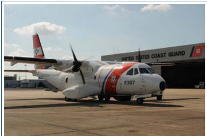
The Coast Guard accepted delivery of the 16th HC-144A Ocean Sentry, joining aircraft currently in operation at Air Stations in Miami, Fla. (pictured above), Mobile, Ala., and Cape Cod, Mass. With an endurance of more than 10 hours, the Ocean Sentry provides enhanced capabilities to carry out key Coast Guard missions, including search and rescue, disaster response, and drug and migrant interdiction. U.S. Coast Guard photo.
