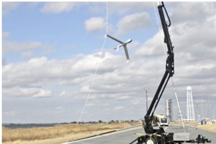
At the conclusion of its seven-hour sortie, the unmanned aircraft “lands” via a “SkyHook” recovery system. On an earlier demonstration aboard a National Security Cutter, the retrieval arm was located to allow the aircraft to fly beside the cutter to enhance crew safety. U.S. Coast Guard photo by Petty Officer 2nd Class Luke Clayton.
