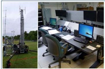
The Rescue 21 Western Rivers lab includes mobile communications equipment that will be used to temporarily replace towers that are damaged or taken offline for maintenance. Dual consoles in the lab help system administrators evaluate new configurations before they are installed in the field. U.S. Coast Guard photos by Hon Leung.
