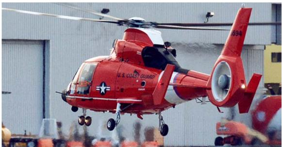
The prototype MH-65E Dolphin takes to the air for the first time in Elizabeth City, North Carolina, Oct. 28. The MH-65E features modernized avionics systems, new sensors and an upgraded flight control system. U.S. Coast Guard photo.
