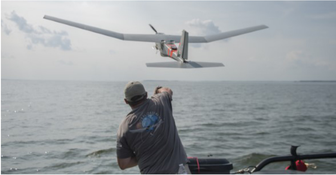
An AeroVironment Puma All-Environment small unmanned aircraft system is launched from Coast Guard Cutter Chock as part of the Research and Development Center's Robotic Aircraft for Maritime Public Safety project. U.S. Coast Guard photo by Petty Officer 2nd Class Luke Clayton.
