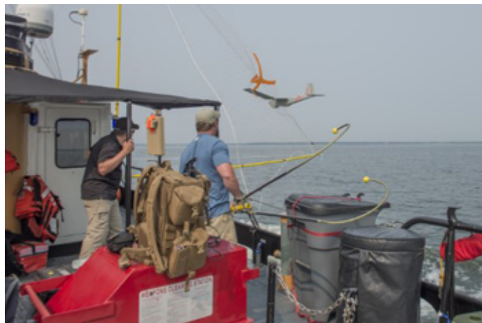
AeroVironment demonstrates an autonomous net capture recovery of the Puma onboard Coast Guard Cutter Chock. The Puma can also be recovered via a water landing. U.S. Coast Guard photo by Petty Officer 2nd Class Luke Clayton.
