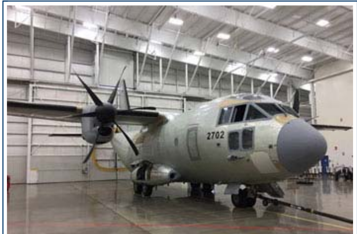
The first C-27J inducted into programmed depot maintenance (PDM), CGNR 2702, awaits a routine overhaul in one of the Heavy Maintenance Facility hangars at Base Elizabeth City, North Carolina. The aircraft was stripped of its paint prior to its arrival and is scheduled to spend a little over a year in PDM. U.S. Coast Guard photo.
