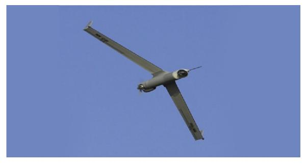
The ScanEagle sUAS will augment the national security cutter's embarked manned helicopter capability with 12 hours of continuous flight time and up to 200 hours of on-station sensor data per month. Courtesy photo.
