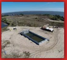
The **JMTF** is located at USCG Sector Mobile in Alabama and provides a relevant maritime test environment that meets (or has appropriate waivers for) all federal, state, and local environmental standards. The **JMTF** includes a burn pan and is the sole national testing facility for in-situ burning research.
