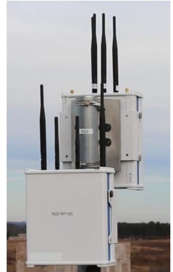
Example of a Passive RF Detection Sensor -DHS C-UAS Tech Guide
