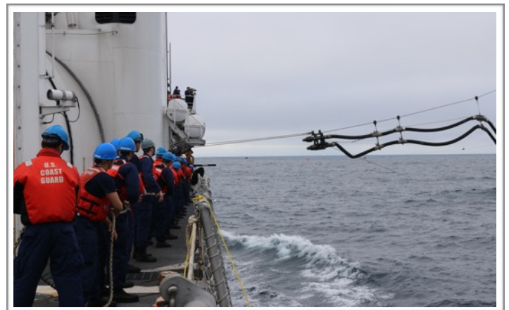
The deck force hauls around to bring the fueling rig over from the oiler.
