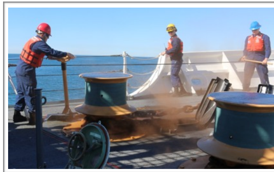
Rust flies as the anchor is let go. This is a normal sight to see after being in port for an extended period.
