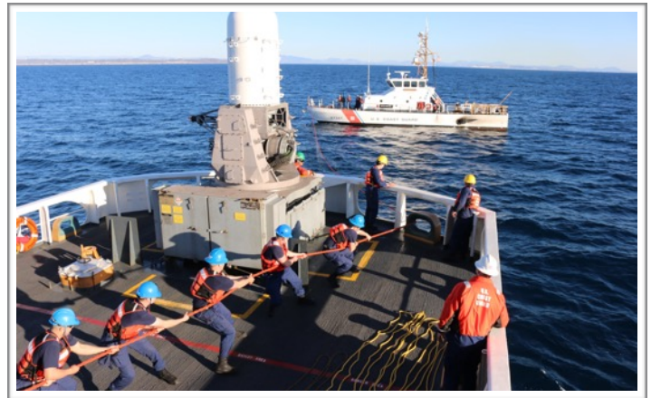
Deck force heaves around on the towing line to bring CGC HADDOCK in closer for a shorter tow as BM3 Mora and BM1 Reagan oversee the evolution..
