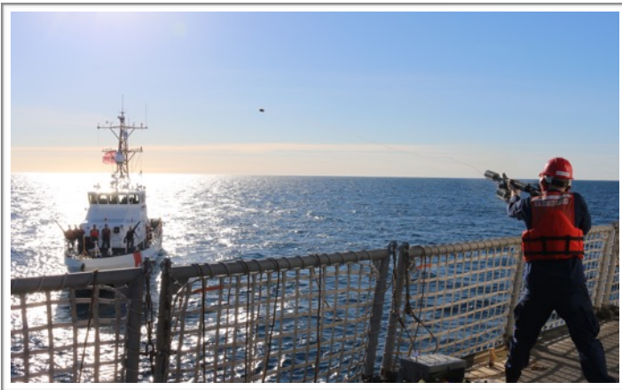
GM3 Lantz uses the line throwing gun to pass the tow line to CGC HADDOCK.
