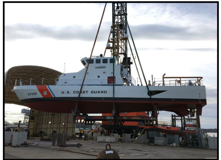
USCGC Chinook, an 87’ Marine Protector Class Patrol Boat, undocks for refloating after completing planned maintenance at the Yard under the 87’ Recurring Depot Availability Project (RDAP). CHINOOK is the 53rd vessel to undergo the RDAP process and the sixth vessel in the fleet class to complete Phase II repair since RDAP began in 2014. The program includes specialized processes, equipment, and labor to reduce schedule variability and minimize costs in order to improve fleet readiness.
