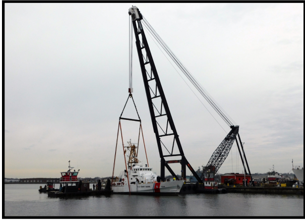
USCGC Key Largo, a 110’ Island Class Cutter is undergoing an emergency dry docking at the CG Yard. The Yard is the only shipyard approved to execute this unique method of craning a 110’ during when dry docked.
