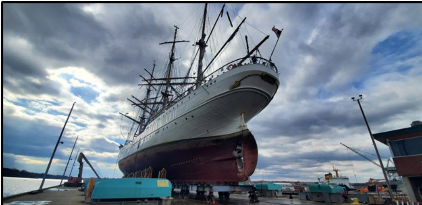
Above: USCGC Eagle was dry-docked at the CG Yard from 24 January 2020 to 22 February 2020 for a planned availability to complete a propeller change-out. Additional work items were completed during the availability to include structural deck renewal, sheet metal fabrication, repairs to the topgallant yardarm, a bearing change-out on the emergency diesel generator and installation of safety rails.
