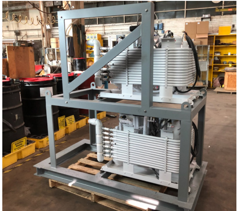
Above: Newly Fabricated HVAC foundation with reconfigured HVAC unit
